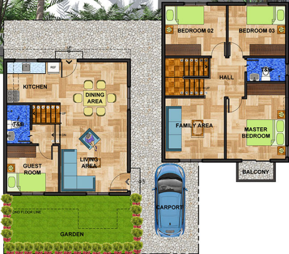
GROUND FLOOR PLAN
